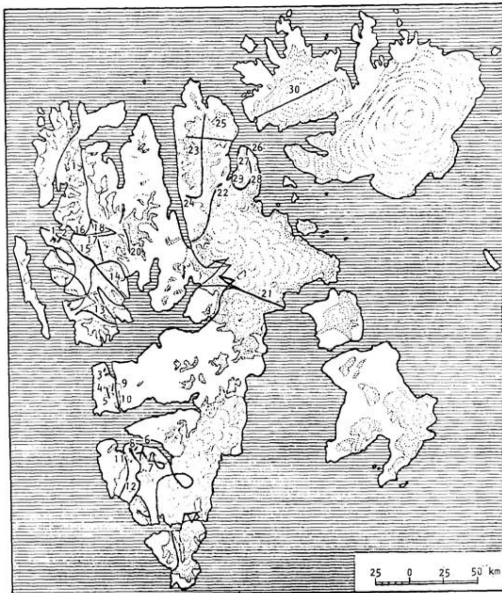
Figure 4. Radio-echo sounding of Svalbard glaciers during 1974-1975 and 1977-1979 field seasons. Lines show the routes of the airborne radio-echo soundings. The figures denote the glaciers whose profiles are shown in figures 5, 6, 7 and 8.
